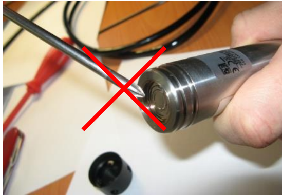
Fig. 60 Incorrect cleaning of the pressure probe
