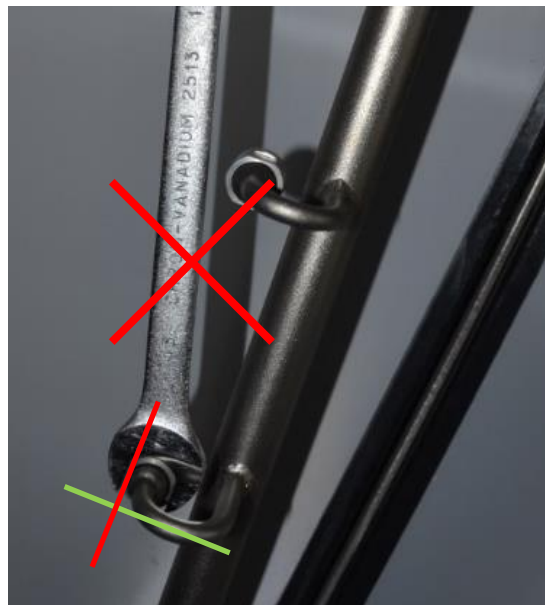
Fig. 57 Incorrect turning of nozzles (see position of the key)
