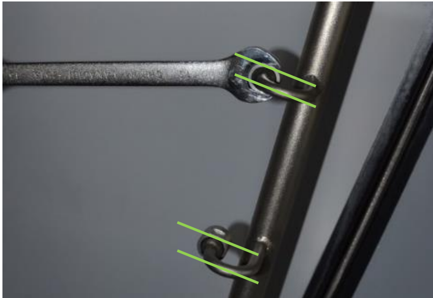
Fig. 56 Correct turning of nozzles (see position of the key)
