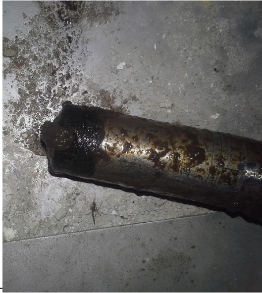
Fig. 48 Dirty pressure probe
