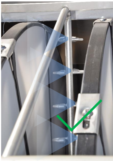
Fig. 46 Correct water jet (shown only on one spray pipe)
