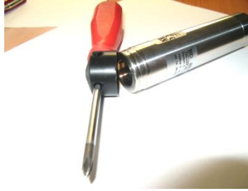
Fig. 59 Correct cleaning of the pressure probe
