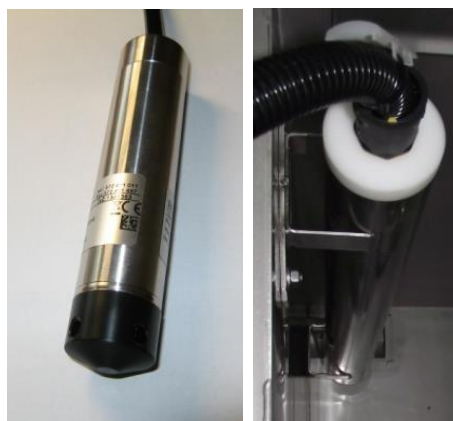
Fig. 19 Pressure probe (detail, in sludge tank)
