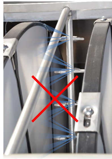
Fig. 47 Incorrect water jet (shown only on one spray pipe)
